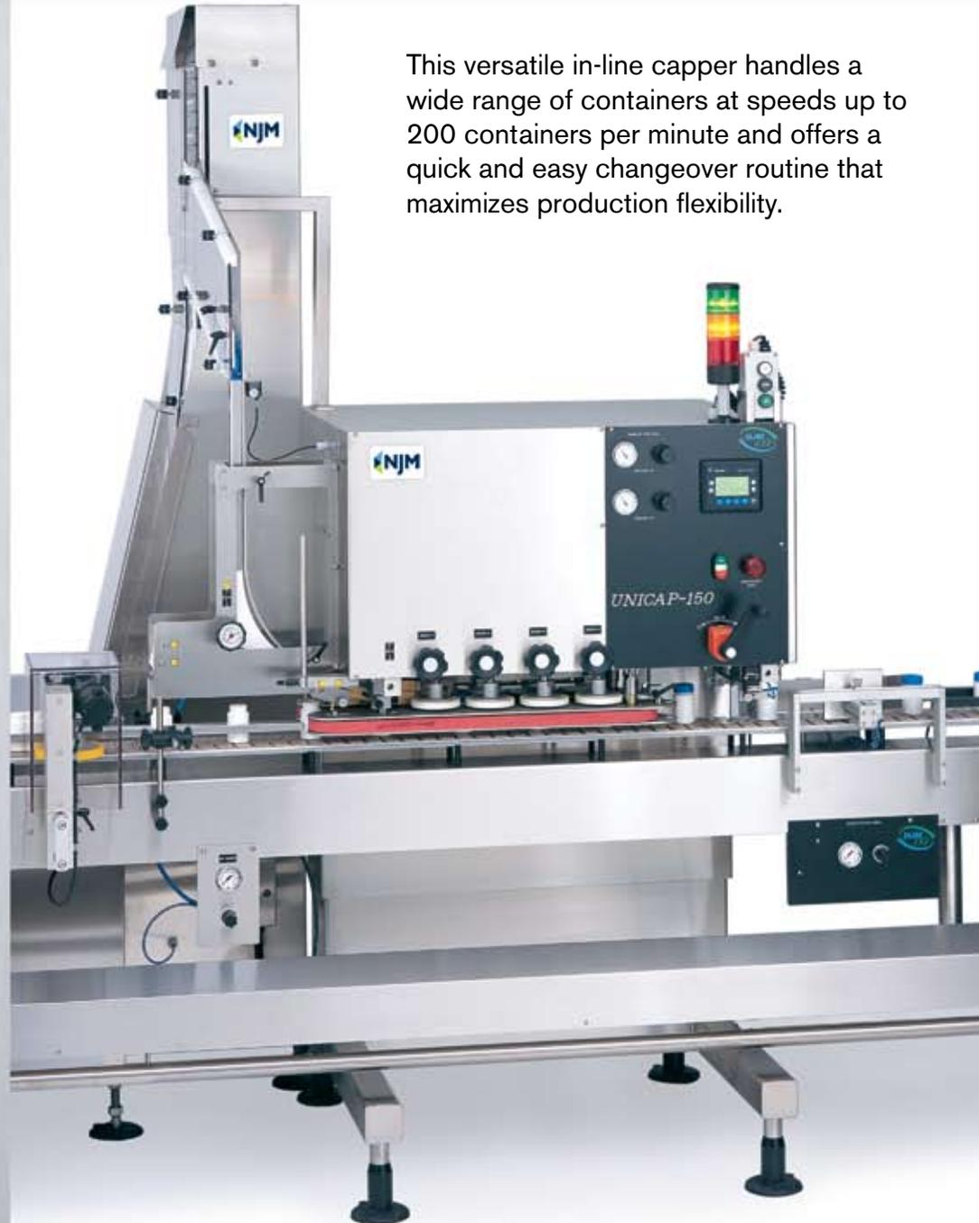
This versatile in-line capper handles a wide range of containers at speeds up to 200 containers per minute and offers a quick and easy changeover routine that maximizes production flexibility.
